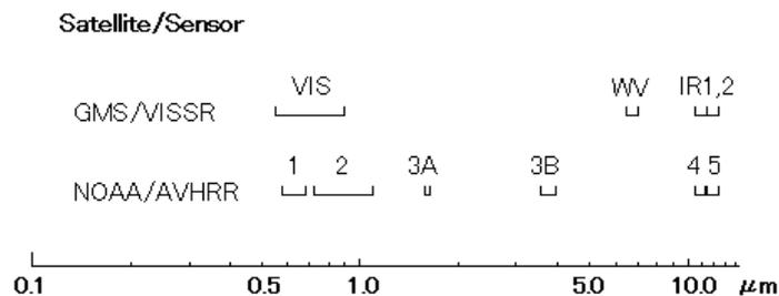
Figure 2 The wavelength bands of NOAA-16/AVHRR and GMS/VISSR sensors
